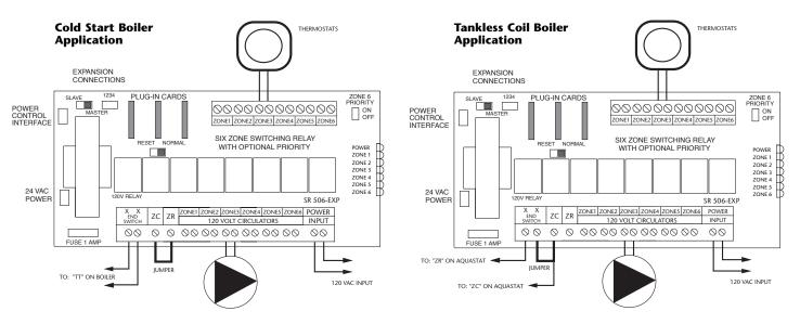
**Warning:** When using Alternative Wiring diagram, wiring instructions must be followed so power originates from the boiler aquastat. Failure to follow these wiring instructions may result in a secondary source of power being connected to the boiler that may activate it under certain circumstances, causing injury or death.
