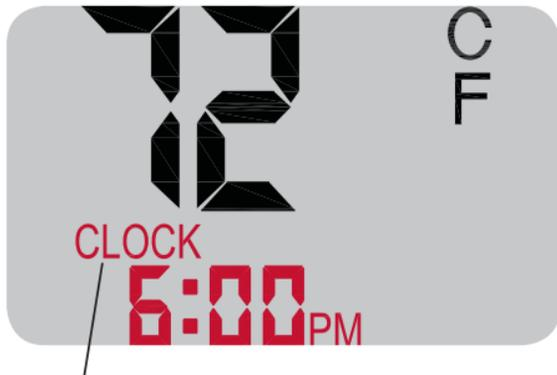
Press ▲ or ▼ buttons in PROG menu until “CLOCK” is flashing.
