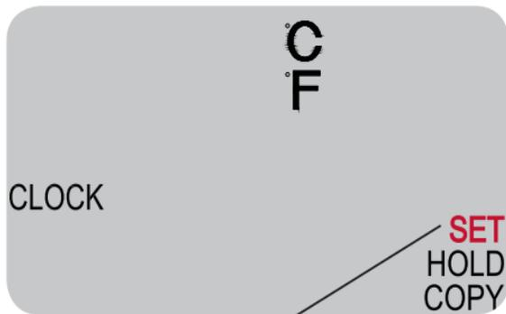
In the PROG menu, press ▲ or ▼ until “SET” is flashing.
