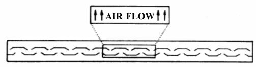
The THRIFTY FLAME STOP FILTER features 2 layers of uniquely formed baffles, secured in a frame. The baffles are arranged to eliminate direct passage of flame or grease through the filter. Grease-laden air is forced to swirl. Accumulation of grease on the baffles is held to an absolute minimum. Drain holes at the bottom of the filter allows rapid runoff to the drain trough.
