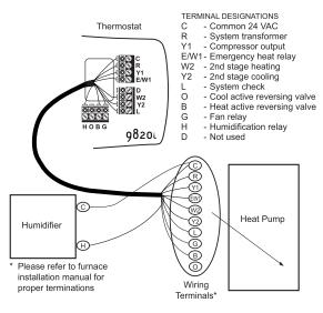
Note: To avoid electrical problems, use the system transformer for both the thermostat and humidifier.
