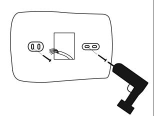
Open the case with a screwdriver. Place in slot and gently pry forward at all four locations.
