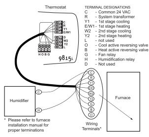
Note: To avoid electrical problems, use the system transformer for both the thermostat and humidifier.
