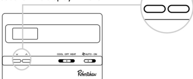
2. Press either the **▼** or **▲** button to adjust the temperature differential up or down.
