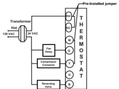
NOTE: Installer must place jumper between "W" and "Y" terminals.
