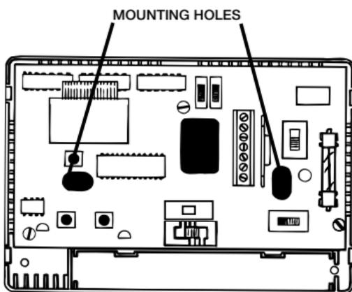
7. Drill the marked holes using a 3/16" drill bit. **NOTE: Enclosed plastic anchors do not require drilled hole for drywall.**
