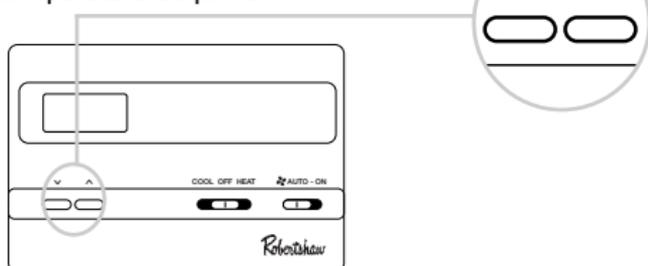
2. Press either the **▼** or **▲** button to adjust the temperature setting either up or down.
