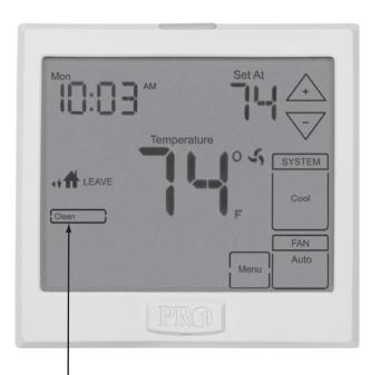
Hold down **CLEAN** for 3 seconds, to reset filter reminder.
