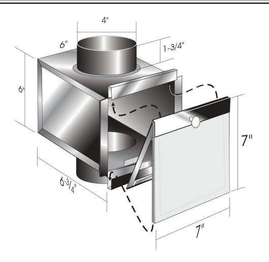
FOR DRYWALL INSTALLATION CEILING OR WALL MOUNTED
