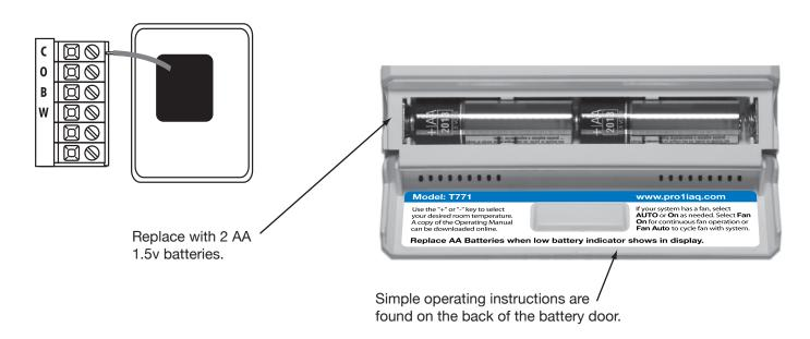
**NOTE:** In applications where the thermostat will see temperatures below 40 degrees it is recommended that 1.5V AA lithium batteries be used instead of alkaline for increased battery life. (Extreme temperatures decrease the life of Alkaline batteries.)
