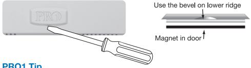
Gently slide a screwdriver into the bottom edge of the badge. Gently turn the screwdriver counter clockwise. The badge is held on by a magnet in the well of the battery door. The badge should pry off easily. Do not use force.
