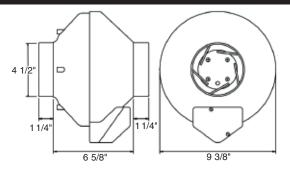
HP2133 – For applications where lower pressure and flow are needed. Record low power consumption of 14-20 watts! Often used where there is good sub slab communication and lower Radon levels.
