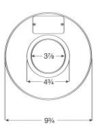
HP175 – The economical choice where slightly less air flow is needed. Often used where there is good sub slab communication and lower Radon levels.
