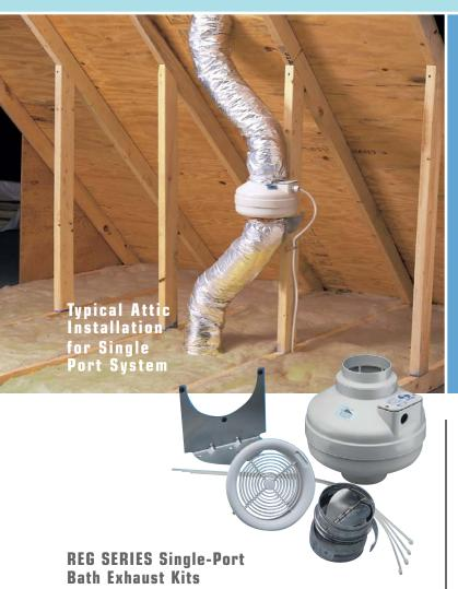
Clear the air in smaller baths and powder rooms with the help of a Fantech REG Series exhaust kit. Each kit includes an inline exhaust fan, mounting bracket, one 4" or 6" grille/collar/damper combination and clamps.
