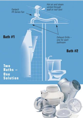
Today's larger master baths require more ventilation than a single exhaust fan in the center of the ceiling. Upgrade to a Fantech two-port bath exhaust kit that ventilates two different areas of a bath from one remote fan. Put one port over the shower and one over the toilet area; or use the kit as shown in the illustration above to ventilate two different baths. Kits include inline fan, mounting bracket, Y-adapter, two 4" or 6" grille/collar/damper combinations and mounting hardware.
