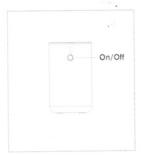
The indicator light will be blue and flash for about one second when the power adaptor is first connected to the purifier, indicating the standby mode. Press the on/off button once to turn on the device; the indicator light will now be a steady blue; the purifier will operate in the default sleep mode (quiet fan speed).
