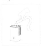
Clean out any remaining dust or hair inside the purifier using a vacuum hose of dry cloth.
