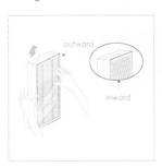
Remove any packing from the new filter elements and take note of the inward and outward sides of the filter element for correct installation.
