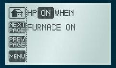
Heat pump protection circuit safeguards the compressor from damage when Stage II heating is located upstream of the evaporator.
