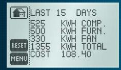
ENERGY WATCH feature acts as an HVAC energy calculator. It monitors kilowatts-per-hour (kWh) consumption and calculates the cost of operating the HVAC system.
