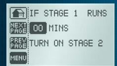
Adjustable "time out" for multistage HVAC systems automatically turns on the second stage for demanding days. This unique timeout feature triggers the second stage for additional heat/cool assistance after the preset time if differential settings are not reached.
