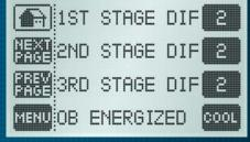
Adjustable differential settings for multistage installations provides precise control of each stage.
