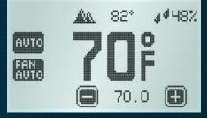
A SIMPLE MODE interface for non-programmable usage is built into Climatouch™ C³. It hides all advanced features, providing a larger display of time, room temperature, humidity and temperature set point.
