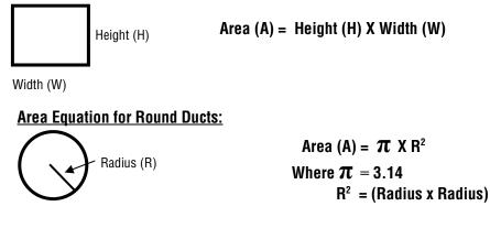
CFM (ft<sup>3</sup>/min) = Air Velocity (ft/min) X Area (in square Inches)
