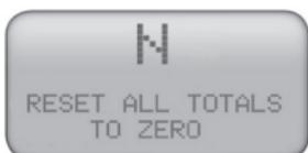
Change the 'N' to 'Y' if you would like to change all of your totals to zero. **NOTE:** This will zero ALL accumulated data totals. You can not specify which totals to zero out. It does not affect the Setup Data (Time, Date, etc.) or the monthly History. Once you have pressed the MODE key, TED takes approximately 1 minute to clear the registers.
