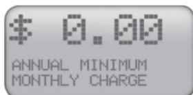
Some utilities, in addition to a charge per kWh, have a minimum charge for electricity. This is typically a flat-fee. Use the ► and ▲ keys to set the rate, then press the MODE Key.
