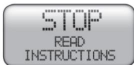
A. Hold the "\$" and ▲ keys down at the same time for 3 seconds and this screen should come up. You are reading the instructions, so go ahead and press the MODE key to go to the next screen.
