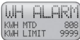
Once set, TED will enter Alarm Mode when the “kWh” figure exceeds the LIMIT set by the user. Example: If the user wishes to be notified when the month-to-date kWh exceeds 1500, the user will have entered 1500 as the LIMIT for the alarm. When 1500 kWh is reached, TED will enter Alarm Mode.
