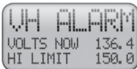
Once set, TED will enter Alarm Mode when the voltage exceeds the LIMIT set by the user. Example: If the user wishes to be notified if the voltage exceeds 125 volts, the user will have entered “130 volts” as the LIMIT for the alarm. If the voltage reaches 130 volts, TED will enter Alarm Mode. High voltage may cause damage to sensitive electrical devices and will also shorten lamp life.
