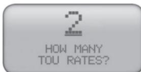
Using the ▲ key, select how many peak rates you have throughout the day. NOTE: If you have a rate of \$.10 from 9-10am and \$.10 again from 3-5pm, this is one (1) rate peak, because it is the same rate even though it is at different times.
