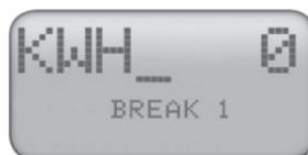
The kWh tiers are shown as "breaks." This is where you put in the upper-value of each tier. Ex: If tier 1 on your bill is from 0 to 150kWh, you would input "150" as Break 1. Use the ► and ▲ keys to input the upper value. Press MODE Key when finished.
