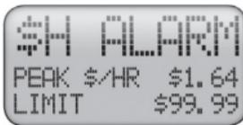
Once set, the alarm will sound when the Cost-Per-Hour "\$/H" figure exceeds the LIMIT set by the user. Example: If the user wishes to be notified when the \$/H exceeds \$1.20, the user will have entered "\$1.20" as the LIMIT for the alarm. Each time \$1.20 is exceeded, TED will enter Alarm Mode.
