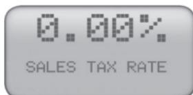
Charged as a percentage calculation of the entire bill. Standard with most utilities. Use the ► and ▲ keys to set the rate, then press the MODE Key
