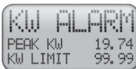
Once set, the alarm will sound when the Power Usage "KW" figure exceeds the LIMIT set by the user. Example: If the user wishes to be notified when the KW exceeds 10.00, the user will have entered 10.00 as the LIMIT for the alarm. Each time 10.00KW is exceeded, TED will enter Alarm Mode.
