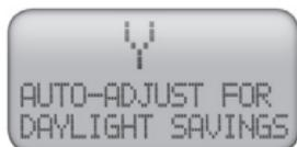
If your locale observes Standard North American Daylight Savings Time, choose “Y” otherwise choose “N.” Use the ▲ key to toggle between “Y” and “N” and then press the MODE key. TED will automatically adjust the time based on the New Daylight Savings Time standard passed by US Congress in 2006.
