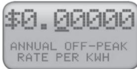
If you make a mistake during this process (or anytime during the Setup Routine), hold the MODE Key down for 3 seconds. It will save all your entries up to this point. To get back into the Setup Mode again to complete your programming, simply hold the \$ and ► keys simultaneously for 3 seconds; press MODE to advance to the area you were wanting to correct or complete. You can override any prior entries at any time.
