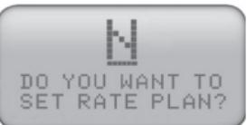
Initially, you will need to input a Rate Plan, so change the 'N' to a 'Y' and press Mode. (If, at a later date you wish to only *CHANGE* your rates while not changing your rate PLAN, press N ).
