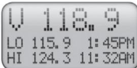
This is the current voltage measured at your electrical panel: 118.9 volts.
