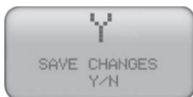
If you have successfully changed/ entered your rates, press the MODE Key. You may change your rates at any time by going through the Setup Routine again. If you want to go back to a field already entered, you will need to go through the Setup Routine again by holding the \$ and ▲ key simultaneously and pressing MODE until you reach the field you wish to modify.
