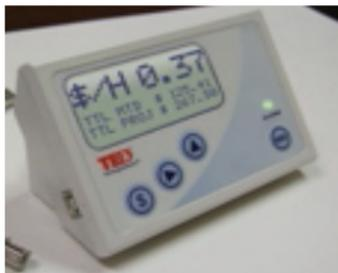
b) One (1) Model 1001 Measuring Transmitting Unit (MTU)
