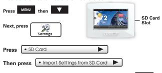
Your thermostat will automatically save your new photos and settings in it's internal memory. When finished, you may remove the SD card. It is not needed for normal thermostat operation.
