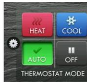
**AUTO-CHANGEOVER MODE** - Pressing the WARMER or COOLER buttons in Auto mode will adjust **both** the heat and cool setpoints simultaneously. To adjust heat and cool setpoints individually, choose HEAT mode to adjust the heat setpoint and COOL mode to adjust the cool setpoint, then return to AUTO mode.
