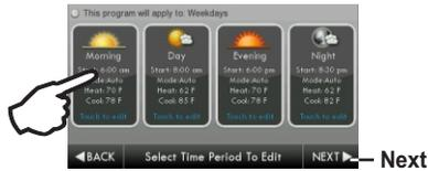
Adjust Mode, Start Time, and Heat and Cool Setpoints to desired settings. The Time Period may also be Enabled or Disabled. Un-check the Enabled box for Time Periods you don't want to use. Press **DONE** when finished.
