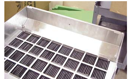
Figure 5: The front of the Solution has four slots to engage the tabs on the dehumidifier bracket. The top two slots are for use when installing on a Phoenix 200 HT and the bottom two are for use on a Phoenix 200 MAX.
