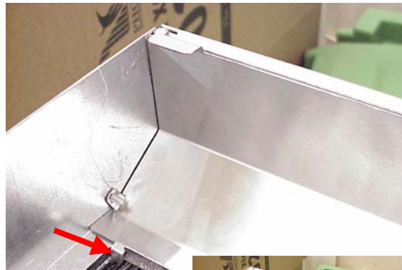
Figure 4: Bracket installed in Phoenix HT using existing fasteners. Note tabs bent down between plastic heat exchanger panels. 200 MAX installation is similar.
