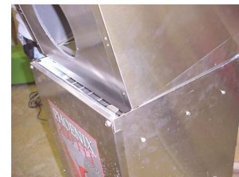
Figure 5: The front of the Solution has four slots to engage the tabs on the dehumidifier bracket. The top two slots are for use when installing on a Phoenix 200 HT and the bottom two are for use on a Phoenix 200 MAX.
