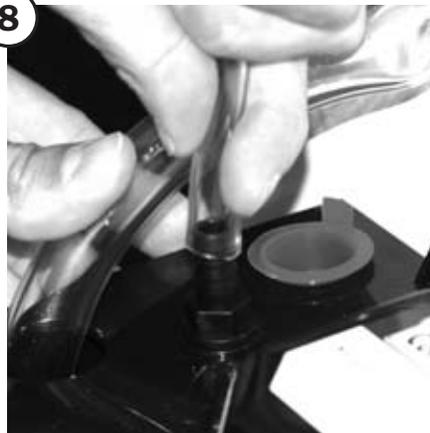
Install the provided drain hose over the condensate pump nipple.
