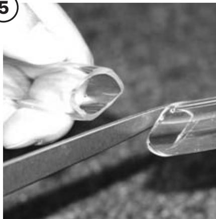
Example of hose cut at a 45° angle. The angle prevents the hose from sealing tight against the bottom of the pump reservoir.
