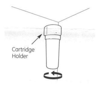
Remove old filter cartridge by grasping and slowly rotating to the left (counterclockwise)
