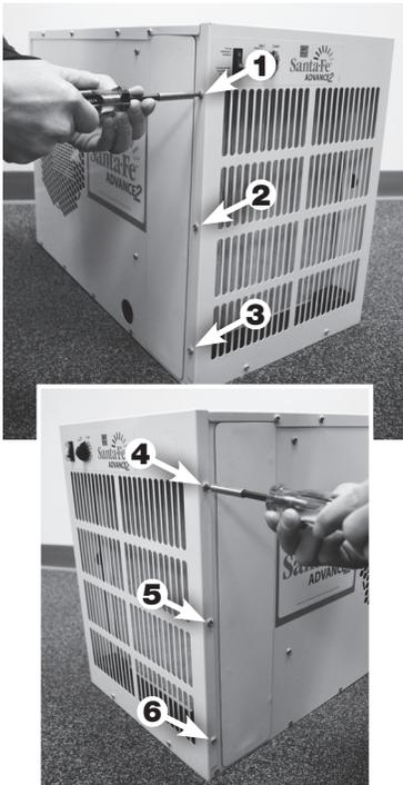
**Step 2:** Place duct kit assembly on dehumidifier and line up holes on assembly with screw holes.
