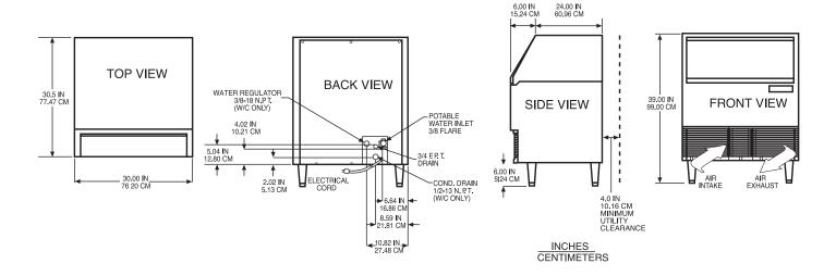
INSTALLATION NOTE: Allow 6" minimum space at back for utility connections.
