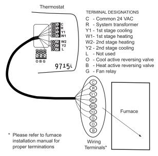
Connect wiring between unit and furnace. For Model 9720i (2H/2C heat pump applications):
