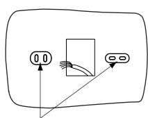
Mark mounting hole locations on wall using unit base as template.
