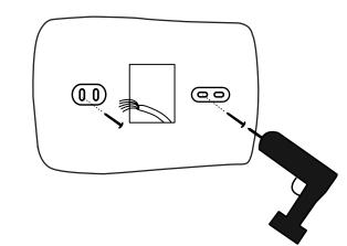
Open the case with a screwdriver. Place in slot and gently pry forward at all four locations.
