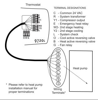
Connect wiring between the thermostat and the indoor sensor (9020i) and the outdoor sensor (9025i), if used. Use twisted pair wiring (22AWG minimum) with a maximum length of 300 feet (or 100m).
