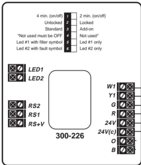
**Note 1:** If jumper is removed, the R terminal may be used to accommodate independent switching circuits.
