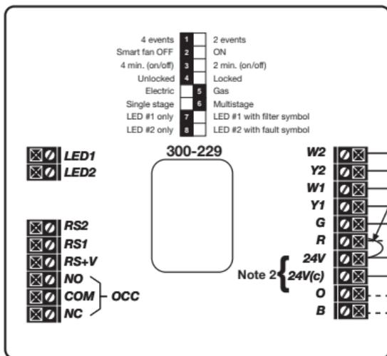
**Note 1:** If jumper is removed, a separate transformer must be used to power the loads.
