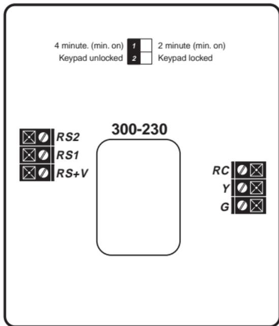
**RC** .....24VAC supply from cooling equipment transformer
