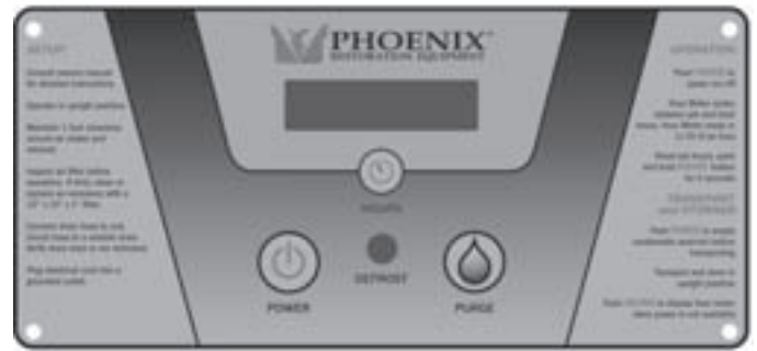
Figure 2: Phoenix R200 control board.
