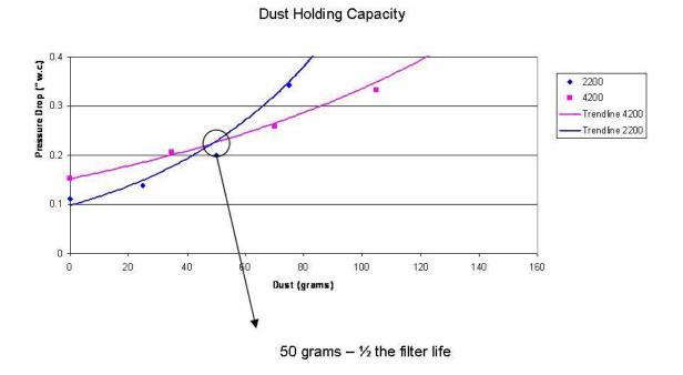
When comparing the resistance to air flow of the Aprilaire 2200 and 4200, the initial pressure drop of the 2200 is lower however after six months (or 50 grams of dust) the pressure drop of the two products is equal. This is due to the depth loading characteristics of the 4200 media. Under normal conditions, 50 grams of dust is about half of the filters life. The remaining life of the media of the 4200 has lower resistance than the 2200.
