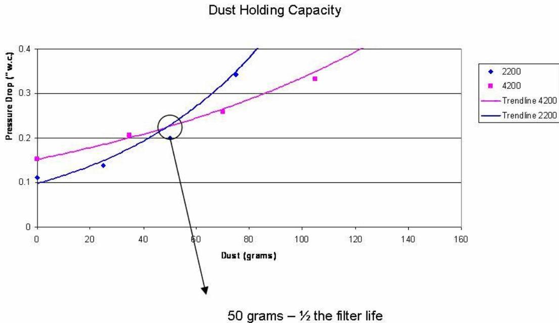
When comparing the resistance to air flow of the Aprilaire 2200 and 4200, the initial pressure drop of the 2200 is lower however after six months (or 50 grams of dust) the pressure drop of the two products is equal. This is due to the depth loading characteristics of the 4200 media. Under normal conditions, 50 grams of dust is about half of the filter's life. The remaining life of the media of the 4200 has lower resistance than the 2200.
