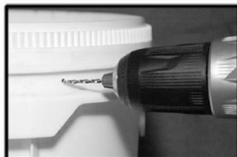
Drill a vent hole, 1/16 inch, in the top section of both buckets
