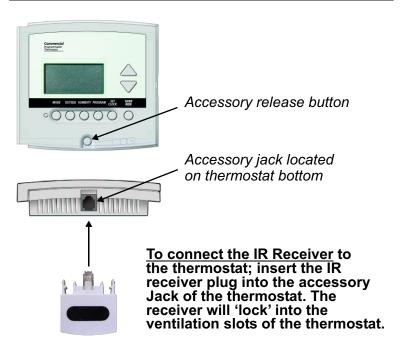
To remove the IR receiver from the thermostat; press and hold the accessory release button while removing the IR receiver from the thermostat's accessory jack.
