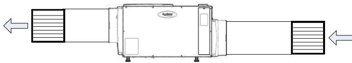
Figure 1 Dehumidifier Ducted Directly
