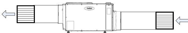
Figure 2 Dehumidifier Ducted Directly
