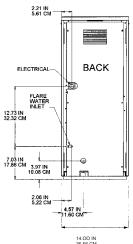
INSTALLATION NOTE: Allow 6" minimum space at sides and back for ventilation and utility connections.
