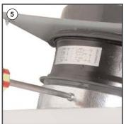
Remove the screw that fixes the elbow to its support on the opposite side. You can now remove the elbow.
