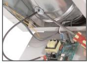
Remove the screw that fixes the elbow to its support.
