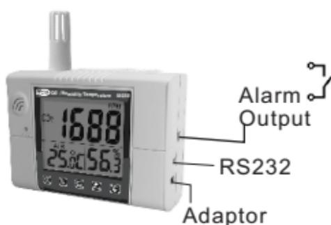
The meter is designed with a relay
