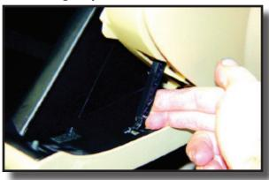
Push in on top of glove box on both right and left sides.
