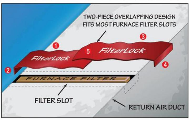
FilterLOCK seals standard furnace air filter slots. Overlapping two-piece design fits up to 25" filters. Built-in magnetic fasteners hold FilterLOCK securely in place on top or side of metal duct.
