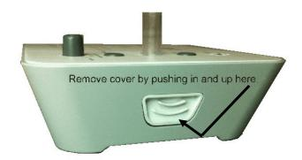
IMPORTANT! Set the Upstream/Downstream switch so that it matches the FILTERSCAN<sup>®</sup> Monitor position with respect to the air filter (that is, OFF for upstream mounting or ON for downstream or differential mounting). The switch can be accessed by removing the front cover of the Monitor.
