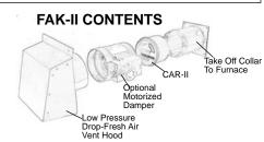
climates, to avoid surface condensation. Duct runs should be as straight and short as possible with a minimum of elbows. If flexible ducting is used, duct run must be no more than 20 feet. Be sure it is properly supported to avoid sags and bends which can restrict airflow. In cold climates, it is important to assure a tight seal between the house and duct vapor barriers, to avoid condensation and ice buildup around the fresh air
