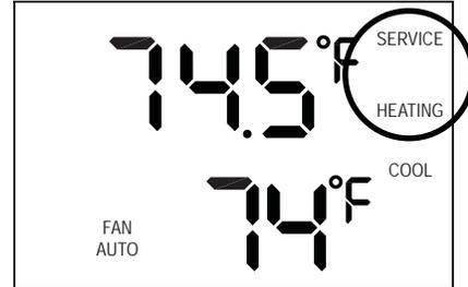
**Example:** When the display shows **SERVICE** and **HEATING** it is time to schedule an appointment to have the heating system maintained.
