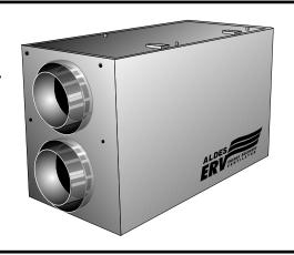
During the winter, an ERV also recovers humidity from the exhaust air to partly humidify the supply air, reducing the need for humidification. The sensible heat performance is similar to an HRV, (Heat Recovery Ventilator) in that it also recovers heat from the exhaust air to temper the fresh outdoor air close to room temperature. (During cold weather, both HRV's and ERV's act to lower indoor humidity by ventilation with drier outdoor air, but an ERV can recover a sig-
