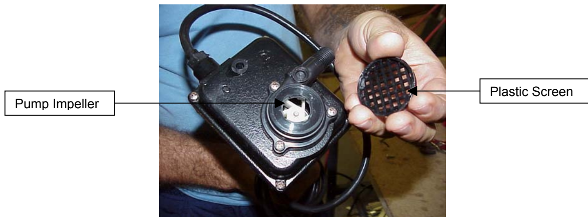
Figure WC-1HP-DHL.06 – Pump
