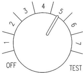
Once your Compustat is installed in the cold air return and internally set to AUTOMATIC, turn the dial to 5 (the standard humidity comfort setting).
