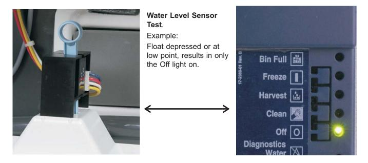
**To Test**: Move the float stick slowly up and down and observe the light display on the controller. **Results**:
