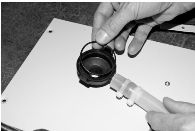
Fig. 8: Make sure O-ring is correctly seated before reassembling impeller.
