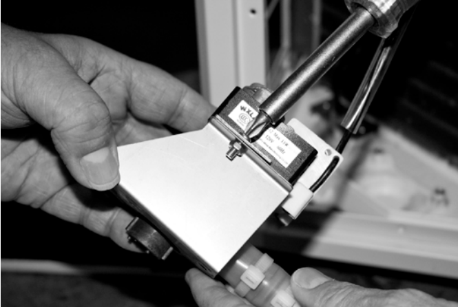
Fig. 6: Remove the pump from the pump bracket.
