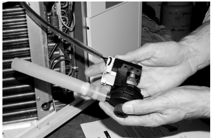
Fig. 9: Reassemble impeller as shown. Make sure electrical cables are oriented in the same direction as the drain tube.
