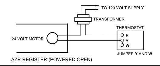
When the AZR Automatic Zone Register<sup>TM</sup> is used with a zone control system, the wires of the register motor should be connected to the proper damper terminals on the zone control panel. The AZR<sup>TM</sup> connects the same as any standard powered closed / spring return open zone damper.
