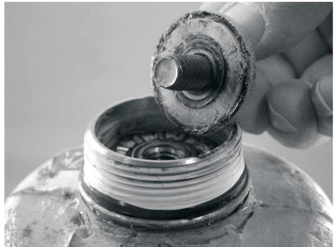
Thrust Washer and Bearing
