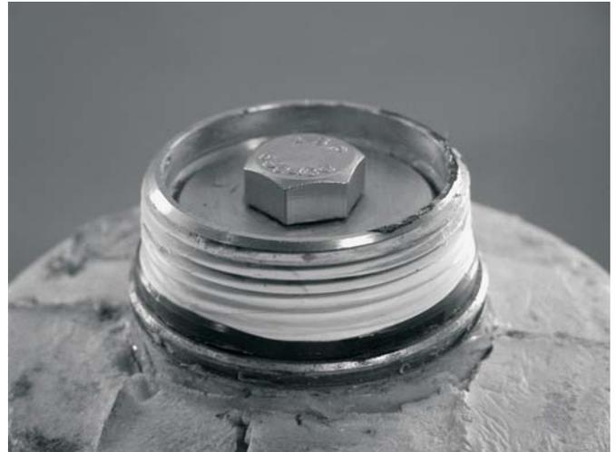
Top of Bearing Thrust Washer
