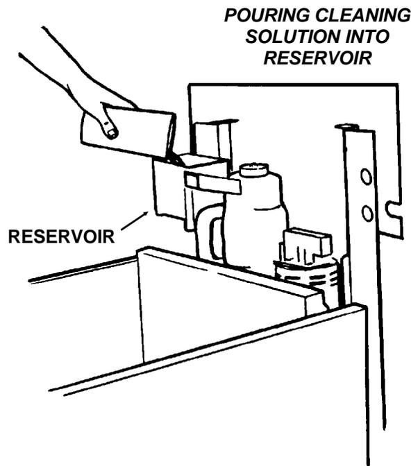
16. Move the master switch to ON, continue to pour cleaning solution into the reservoir until it has all been used.
