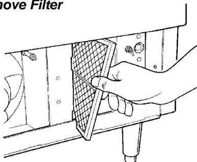
or, if torn or so dirty it can't be cleaned, replace with a new filter.
