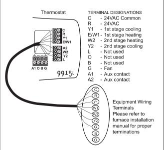
Connect wiring between unit and heat pump. For Model 9920i (2H/2C heat pump applications).
