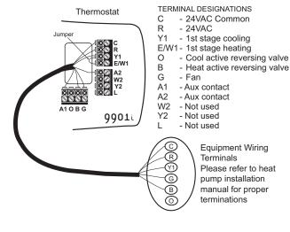
Connect wiring between unit and furnace. For Model 9915i (2H/2C furnace applications).
