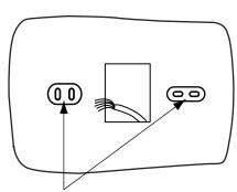
Mark mounting hole locations on wall using unit base as template.
