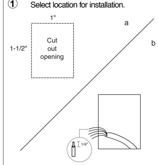
Remove 1/4" of insulation from end of each wire
