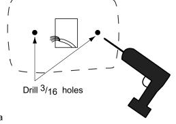
Drill 3/16" holes at marked locations on
