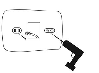
(12) Connect wiring between the thermostat and the indoor sensor (9020i) and the outdoor sensor (9025i), if used. Use twisted pair wiring (22AWG minimum) with a maximum length of 300 feet (or 100m).
