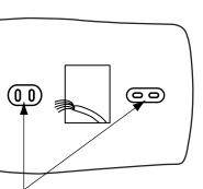
Mark mounting hole locations on wall using unit base as template.
