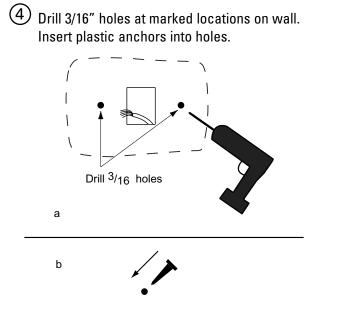
Press anchors into holes until flush.
