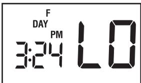
This condition could occur from the system being turned off during a cold weather period or upon installation when the thermostat has been stored for a long period of time in a cold vehicle or location prior to being installed. The thermostat should be allowed to warm up prior to installation in order to provide proper heating control once installed.
