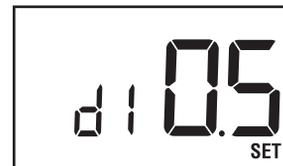
1. In normal operating mode, press and hold the **RETURN** button for 4 seconds. The LCD display will show "d1 X", where "X" equals the °F / °C differential setting. This is the current temperature differential setting.
