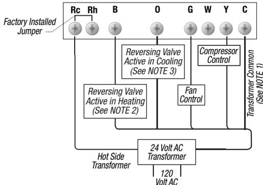
**NOTE:** 1. Transformer Common connection not required for battery-only operation of thermostat. 2. For units requiring reversing valve to be energized during heating, connect reversing valve to B terminal. 3. For units requiring reversing valve to be energized during cooling, connect reversing valve to O terminal.
