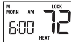
To unlock the keypad, press and hold the **▲** and **▼** buttons together at the same time for 1 second. The **LOCK** segment will disappear and the keypad will become unlocked.
