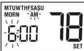
2. Press the **PROG** button to enter Program setting mode. The **MORN** set point of the Whole Week Quick Program Group will be displayed. The display will show **M, TU, W, TH, F, SA, SU**, indicating the whole week is being programmed. The hour portion of the set point time and the **AM/PM** indicator will be flashing.
