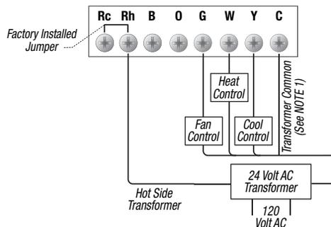
**NOTE:** 1. Transformer Common connection not required for battery-only operation of thermostat. 2. For Heating or Cooling Only System, ignore opposite connection. 3. For 2-Wire 24 Volt AC or 250 mv - 750 mv Millivolt Heating Systems, ignore cooling connection and fan control.
