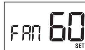
1. In normal operating mode, press and hold the **RETURN** button for 4 seconds. Press **RETURN** again until "FAN XX" is displayed where "XX" is the fan delay time in seconds.
