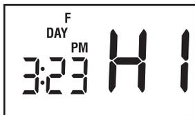
This condition could occur from the system being turned off during an exceptionally warm period or upon installation when the thermostat has been stored for a long period of time in a warm vehicle or location prior to being installed.
