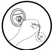
NOTICE OF CAUTION! DO NOT disconnect the wires from the existing thermostat before reading these instructions. The wires must be labeled prior to removal to ensure proper connection.
