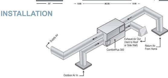
The ComfortPlus 300 is typically installed as shown with its own return air and supply ducts. The supply air duct is branched to two or three supply air ducts servicing main rooms of the home. The ComfortPlus 300 is controlled by a separate humidistat and will cycle on and off to control humidity independently of the main A/C system.
